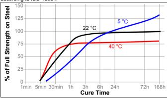
The rate of cure will depend on the temperature. The graph below shows the breakloose strength developed with time at different temperatures vs @ 23°C on 3/8" NPT malleable steel tees and steel plugs, pretorqued to 23N·m and tested according to ASTM D6396.
